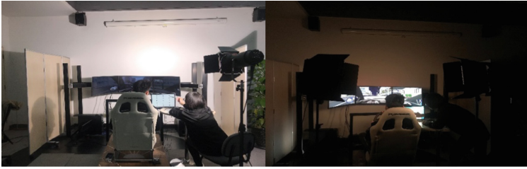
Fig. 3. Overall view of the simulator-daytime lighting (left), nighttime lighting (right)
