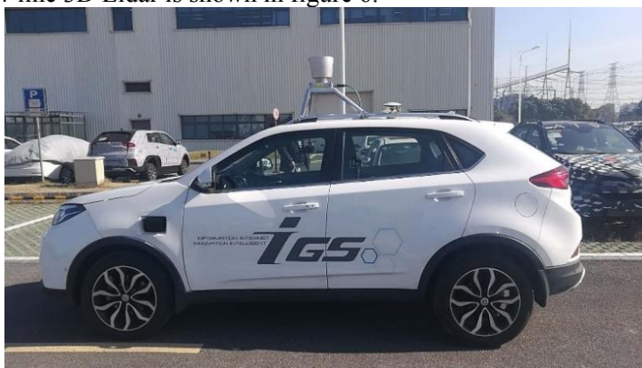
Figure 6. the test vehicle equipped with the 64-line 3D Lidar.
