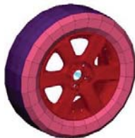
Figure 3. Tire finite element model.
