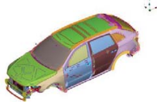
Figure 1. Finite element model of decorative body.
