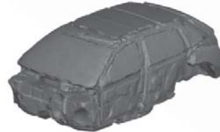
Figure 4. Finite element model of the acoustic cavity in the car.
