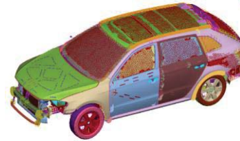
Figure 6. Finite element model of sound-structure coupling of the vehicle.
